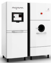
a. EBM equipment b. Examples of components in Ti alloy elaborated by additive manufacturing
