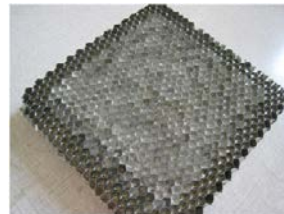
Fig.2 : example of a hosting structure for a PCM wax : a aluminum honeycomb.
